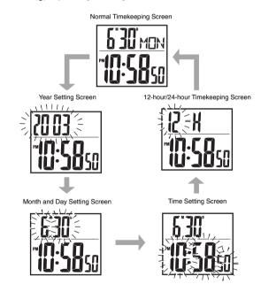
2. While the screen you want is on the display, use the **Alarm Time Set buttons (③)** to change the digits that are flashing.
